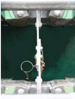
图 2 构件加载照片 Fig.2 Photo of the specimens under load
