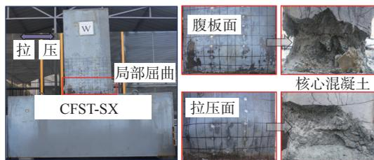
(c) 试件CFST-SX( $B=600$  mm), 网格尺寸 $50\text{ mm}\times 50\text{ mm}$
